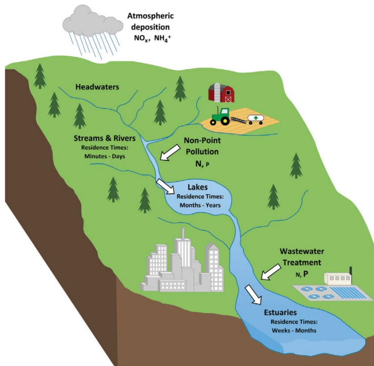
Figure 5.2 A watershed unit includes the land and the stream and riverine network it drains. It is delineated by a drainage divide which is land formation with the highest elevation from which headwaters originate. Included also are non-point and point sources of nutrients leading to estuaries and coastal waters. (Source: Wurtsbaugh et al. 2019)
