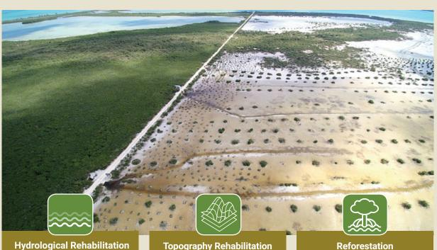
**Objective:** Restore the hydrology by reconnecting water flows with freshwater and/or marine brackish sources in the degraded zone, in order to restore the flooding level, duration, and frequency that enables the restoration of physicochemical conditions of water and soil.
