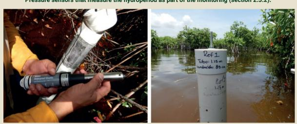
Pressure sensors that measure the hydroperiod as part of the monitoring (section 2.3.2).
