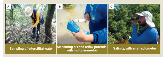
**Figure 2.27** – Sampling of interstitial water (A), measuring pH and redox potential with multiparametric (B), and salinity, with a refractometer (C).
