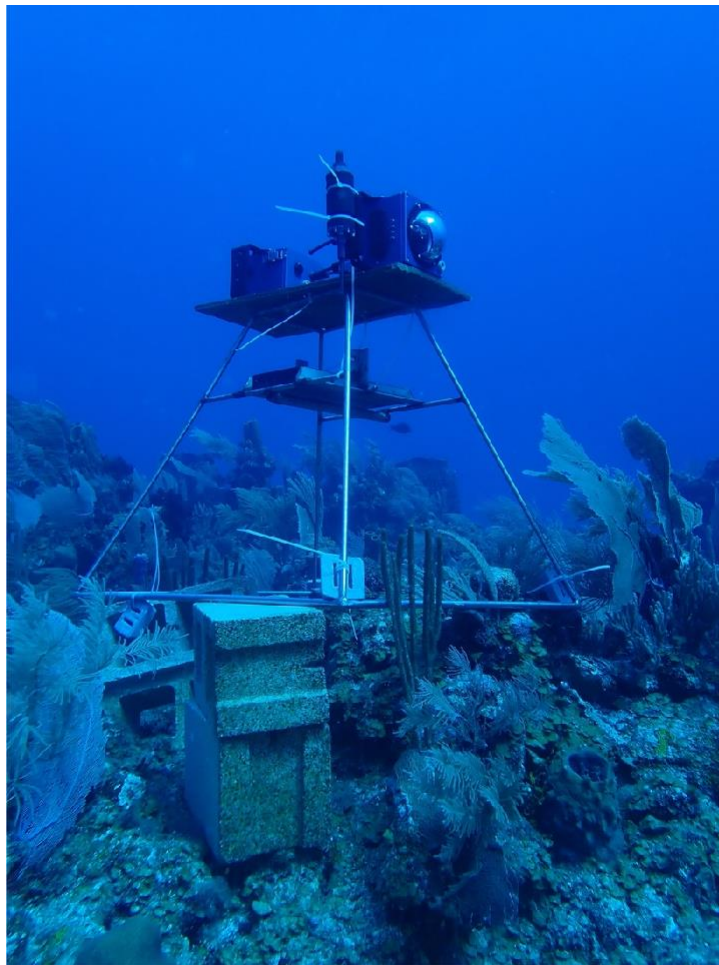
Figure 8. Three hundred and sixty-degree camera (360°) mounted on BRUV at Tiger Bank FSA, Glover's Reef Atoll, Belize. Credit:M. Phillips/WCS.
