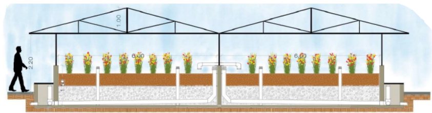
Figure 7: Drying beds with plants. Source: BORDA Las Américas (2022)
